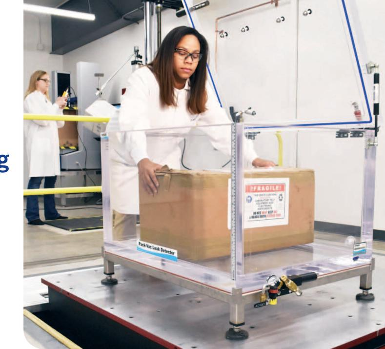
**Distribution Testing:** No matter how or where your product is shipped, Eurofins Medical Device Testing's state-of-the-art distribution testing equipment can simulate the stresses of shipping on products. Standard ASTM and ISTA distribution cycles, as well as custom programmes, can be performed that simulate stacking, manual handling, and vibrations associated with various forms of transport, as well as pressure changes that can be seen during air or mountainous product transportation.
